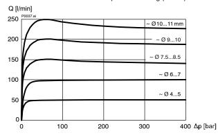
Q = f ( $\Delta$ p) Flow rate - Pressure drop characteristic at the mid-range compensator setting (12 bar)
