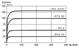
Q = f ( $\Delta$ p) Flow rate - Pressure drop characteristic at the maximum compensator setting (16 bar)
