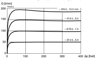
$\Delta p$  = f (Q) Pressure-drop characteristic (control  $\Delta p$ , 2 $\rightarrow$ 1) (port 3 completely unloaded)
