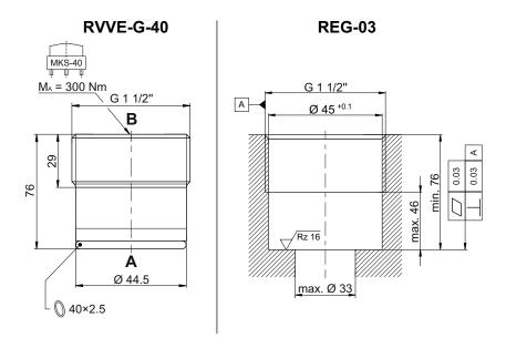
**RVVE-G-40** = check valve / screw-in cartridge valve **REG-03** = dimension of the cavity for screw-in cartridge RVVE-G-40
