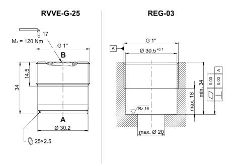
**RVVE-G-25** = check valve / screw-in cartridge valve **REG-03** = dimension of the cavity for screw-in cartridge RVVE-G-25
