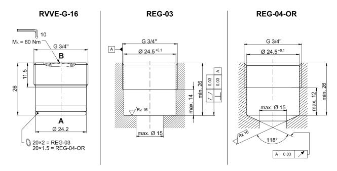
**RVVE-G-16** = check valve / screw-in cartridge valve **REG-03 / REG-04** = dimension of the cavity for screw-in cartridge RVVE-G-16
