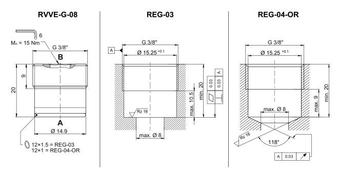
RVVE-G-08 = check valve / screw-in cartridge valve
