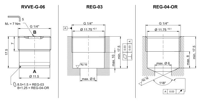
**RVVE-G-06** = check valve / screw-in cartridge valve **REG-03 / REG-04** = dimension of the cavity for screw-in cartridge RVVE-G-06
