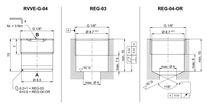
**RVVE-G-04** = check valve / screw-in cartridge valve **REG-03 / REG-04** = dimension of the cavity for screw-in cartridge RVVE-G-04
