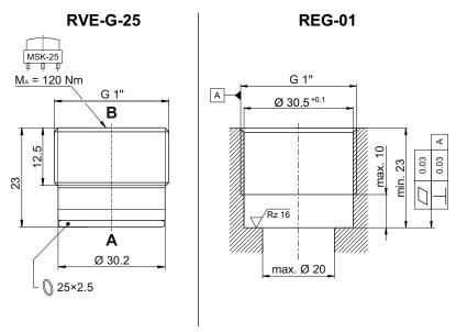
**RVE-G-25** = check valve / screw-in cartridge valve **REG-01** = dimension of the cavity for screw-in cartridge RVE-G-25
