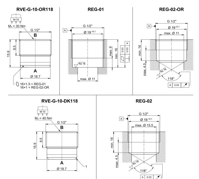
**RVE-G-10** = check valve / screw-in cartridge valve **REG-01** = dimension of the cavity for screw-in cartridge RVE-G-10 **REG-02** = dimension of the cavity for screw-in cartridge RVE-G-10 **REG-02-OR** = dimension of cavity type for screw-in cartridge RVE-G-10 **1** = sealing edge for metal-to-metal sealing
