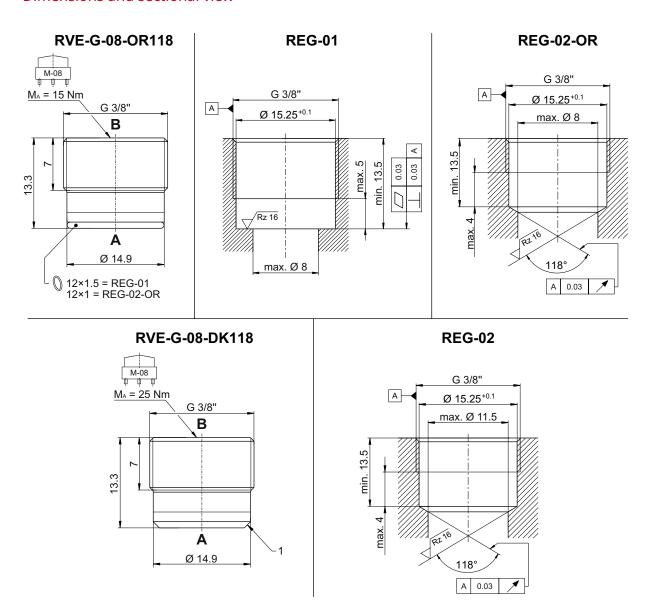
**RVE-G-08** = check valve / screw-in cartridge valve
