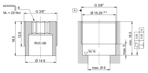
**RVC-06** = spring-loaded check valve / slip-in cartridge valve
