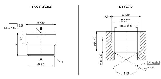
RKVG-G-04 = check valve / screw-in cartridge valve REG-02 = dimension of the cavity for screw-in cartridge RKVG-G-04 RKVG-G-04 1 = sealing edge for metal-to-metal sealing The dimensions specified apply to the mounted state.
