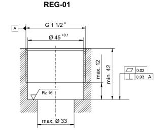
**RKVE-G-40-\_-VD** = check valve / screw-in cartridge valve **REG-01** = dimension of the cavity for screw-in cartridge RKVE-G-40-\_\_-VD **1** = sealing edge for metal-to-metal sealing
