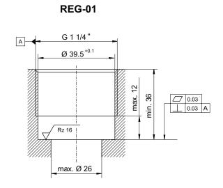
**RKVE-G-32-\_-VD** = check valve / screw-in cartridge valve **REG-01** = dimension of the cavity for screw-in cartridge RKVE-G-32-\_\_-VD **1** = sealing edge for metal-to-metal sealing
