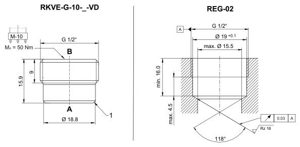
**RKVE-G-10-\_-VD** = check valve / screw-in cartridge valve **REG-02** = dimension of the cavity for screw-in cartridge RKVE-G-10-\_\_-VD **1** = sealing edge for metal-to-metal sealing The dimensions specified apply to the mounted state.
