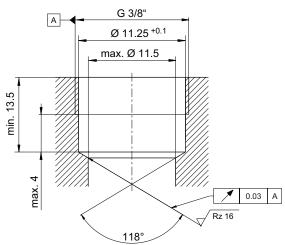
RKVE-G-08-\_-VD = check valve / screw-in cartridge valve
