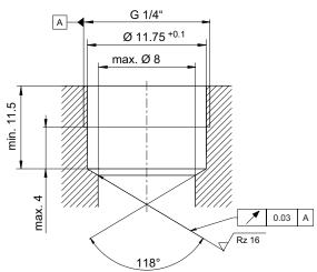
RKVE-G-06-\_-VD = check valve / screw-in cartridge valve
