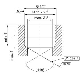
**RKVE-G-06-02-KB** = check valve / screw-in cartridge valve **REG-05-E** = dimension of the cavity for screw-in cartridge RKVE-G-06-02-KB **1** = sealing edge for metal-to-metal sealing
