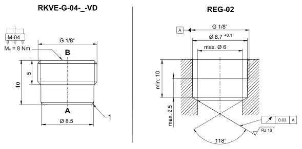
**RKVE-G-04-\_\_-VD** = check valve / screw-in cartridge valve **REG-02** = dimension of the cavity for screw-in cartridge RKVE-G-04-\_\_-VD **1** = sealing edge for metal-to-metal sealing The dimensions specified apply to the mounted state.
