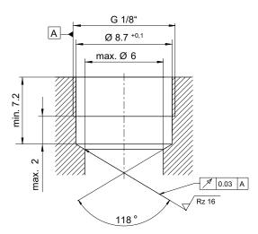
**RKVE-G-04-02-KB** = check valve / screw-in cartridge valve **REG-05-E** = dimension of the cavity for screw-in cartridge RKVE-G-04-02-KB **1** = sealing edge for metal-to-metal sealing
