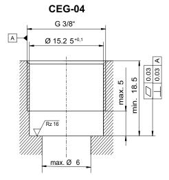
**RKVC-06** = spring-loaded check valve / slip-in cartridge valve **CEG-01, CEG-02 and CEG-03** = dimension of the cavity for screw-in cartridge RKVC-06 **ESH-08** = threaded mounting sleeve for RKVC-06 **CEG-04** = dimension of the cavity for threaded mounting sleeve ESH-08
