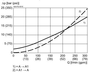
$\Delta p = f(Q)$  Pressure drop-flow rate characteristic
