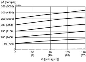
p = f(Q) Pressure - Flow rate characteristic (100 bar)
