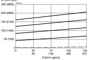
p = f (Q) Pressure - Flow rate characteristic (40 bar)
