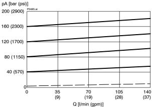
p = f(Q) Pressure - Flow rate characteristic (40 bar)
