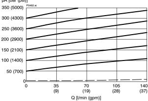
p = f (Q) Pressure - Flow rate characteristic (160 bar) pA [bar (psi)]
