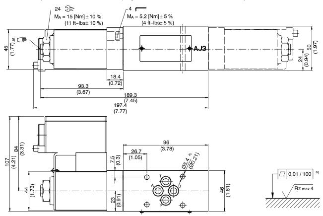
2/2 solenoid operated directional seat valve (double-solenoid model)
